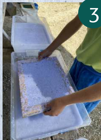
3 Submerge your paper making screen and lift to create an even layer
